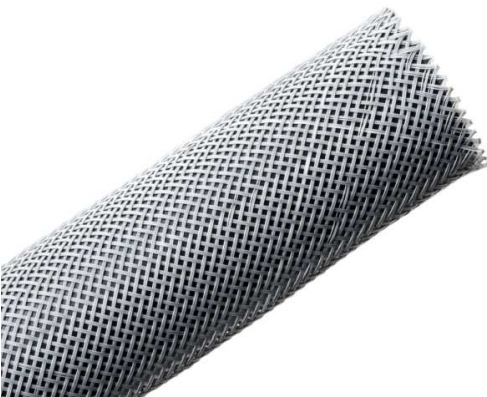
Braided Sleeving, Expandable, Flame Retardant, 0.75" Dia, PET, Gray, 75 ft/reel
