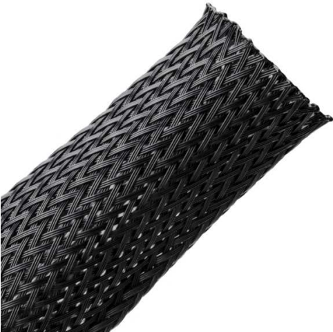
Braided Sleeving, Expandable, 1" Dia, PA66 Monofilament, Black, 50 ft/reel
