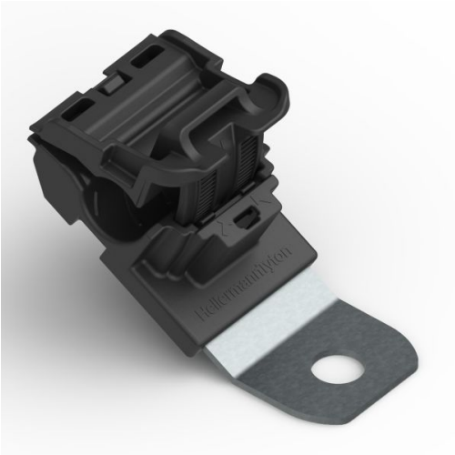
Ratchet P-Clamp, 0.24 - 0.54" Bundle Dia, 30° Long, .26" Hole Dia, PA66HIRHSUV/SS304, Black, 200/ctn
