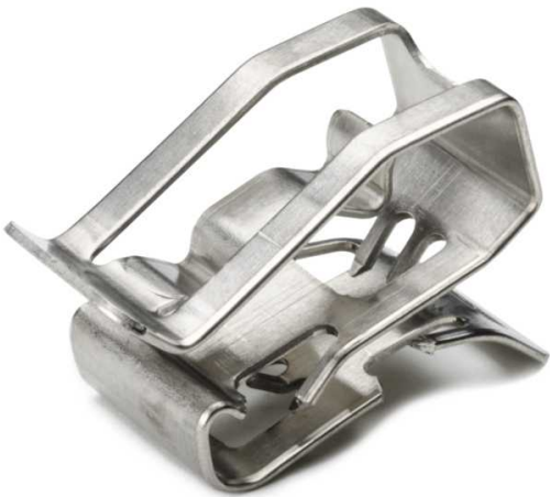
Heavy Duty Metal Edge Clip, 1–3mm Panel Thickness, 5–7.6mm Cable Range, SS304, 100/bag
