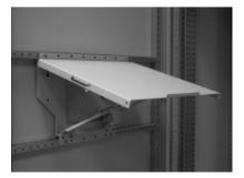
Mounts to internal door channel using 1 or 2 door support rails (sold separately) or directly to a door/side panel using supplied hardware. Can be easily positioned at various heights.
