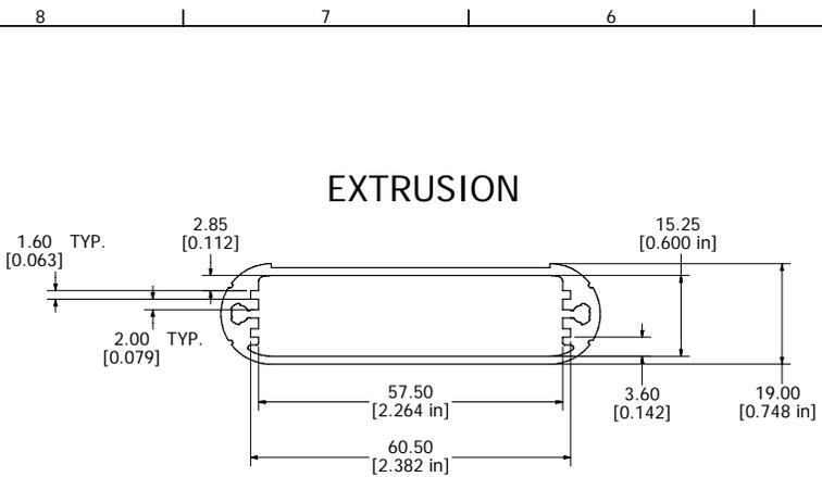
Extrusion designed for 60mm wide x 80mm long PCBs.
