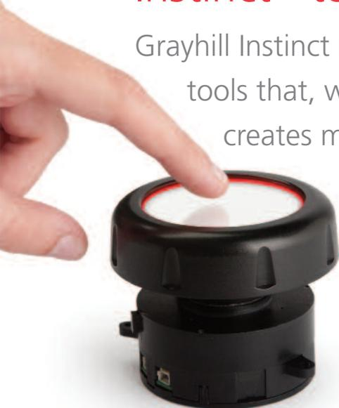
The Multi-Touch Ring Encoder combines a touchpad with multi-touch tracking, an optical encoder and pushbutton into one easy-to-use device. By combining gesture recognition technology with a ring encoder, we provide the ultimate in input flexibility. Menu search, selection, navigation and much more are all in one user interface that can be easily integrated into future devices.
