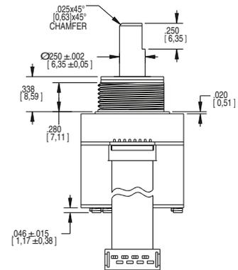
PANEL SEAL GASKET NOT SHOWN TO ILLUSTRATE MOUNTING SURFACE
