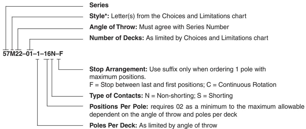
\* All rotary switches that are required to have military designated markings and testing adhering to MIL-DTL-3786 are to be ordered by specifying the military part number identified on the appropriate slash sheet.
