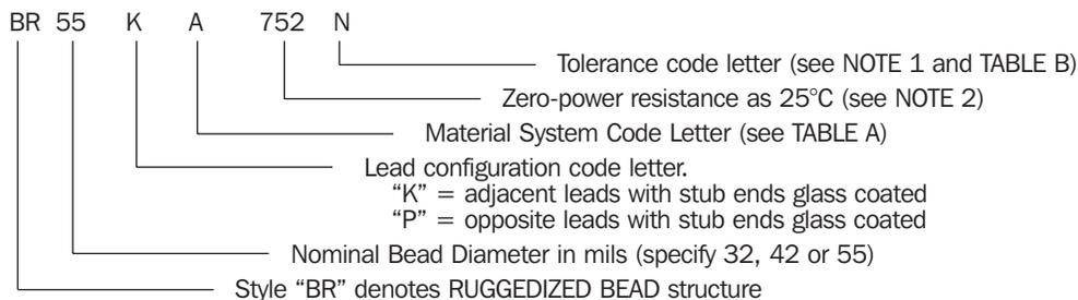
**NOTE 1:** Special tolerances are available on request. Consult factory for special resistance tolerances, non-standard resistances and/or non-standard temperatures.
