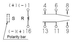
S shows the polarity of set position R shows the polarity of reset position
