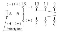
S shows the polarity of set position R shows the polarity of reset position
