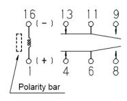
Single Coil Latching type (Top view reset position)
