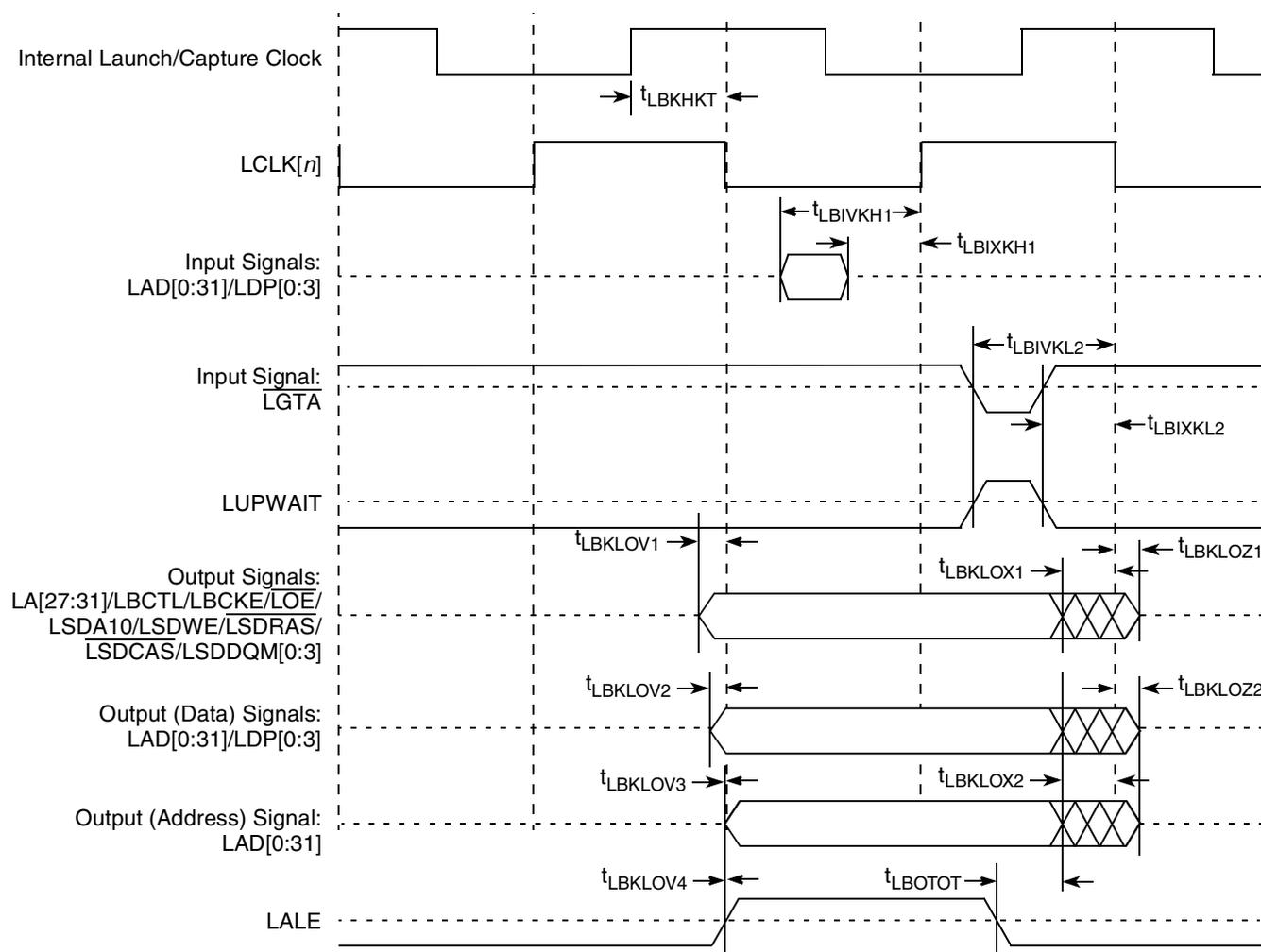
Figure 24. Local Bus Signals (PLL Bypass Mode)
