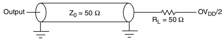
Figure 33. I<sup>2</sup>C AC Test Load
