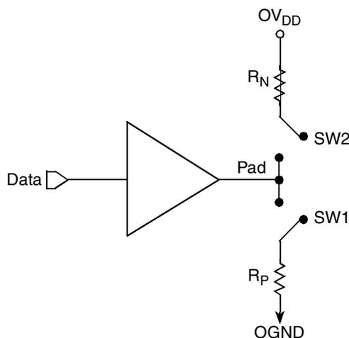
Figure 60. Driver Impedance Measurement
