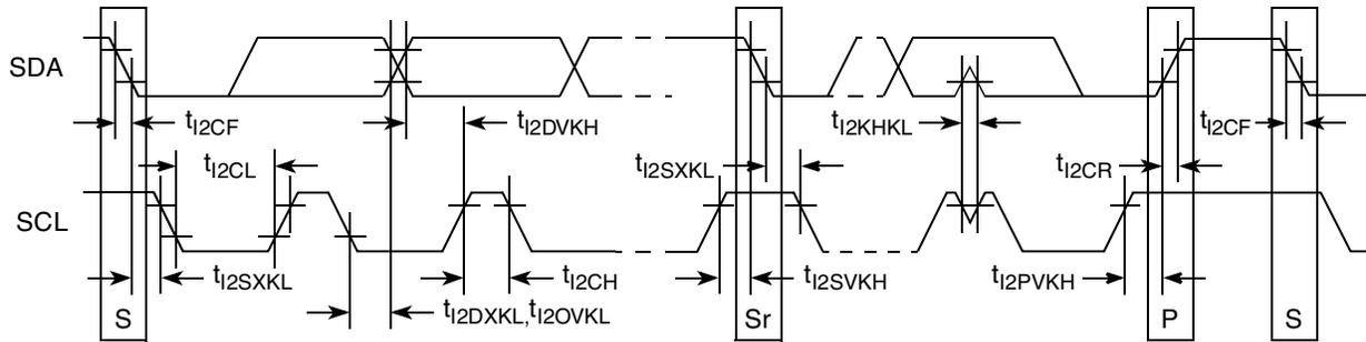
Figure 34. I<sup>2</sup>C Bus AC Timing Diagram
