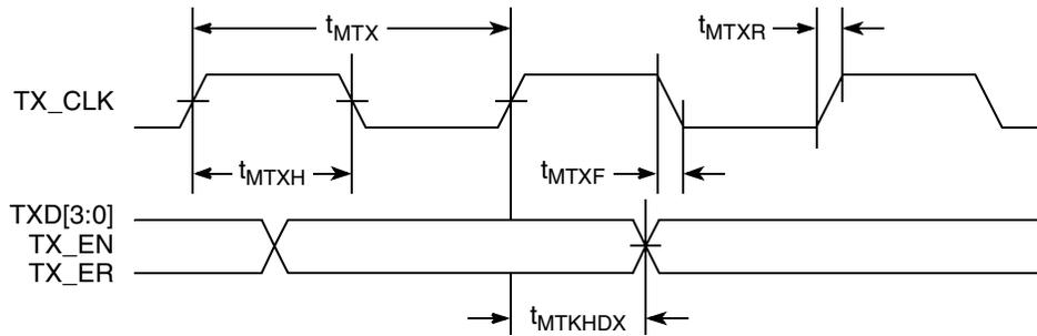
Figure 11. MII Transmit AC Timing Diagram
