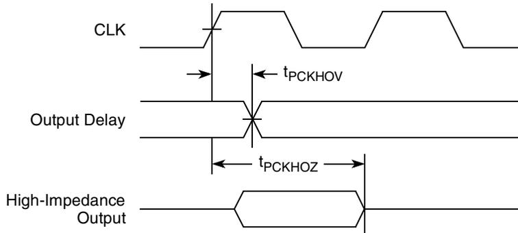
Figure 37. PCI/PCI-X Output AC Timing Measurement Condition
