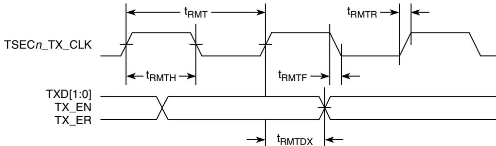
**Figure 18. RMIITransmit AC Timing Diagram****8.2.7.2 RMIITransmit Receive AC Timing Specifications****Table 34. RMIITransmit Receive AC Timing Specifications**
