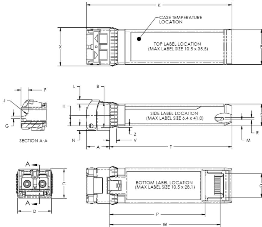
Figure 2. Mechanical Dimensions
