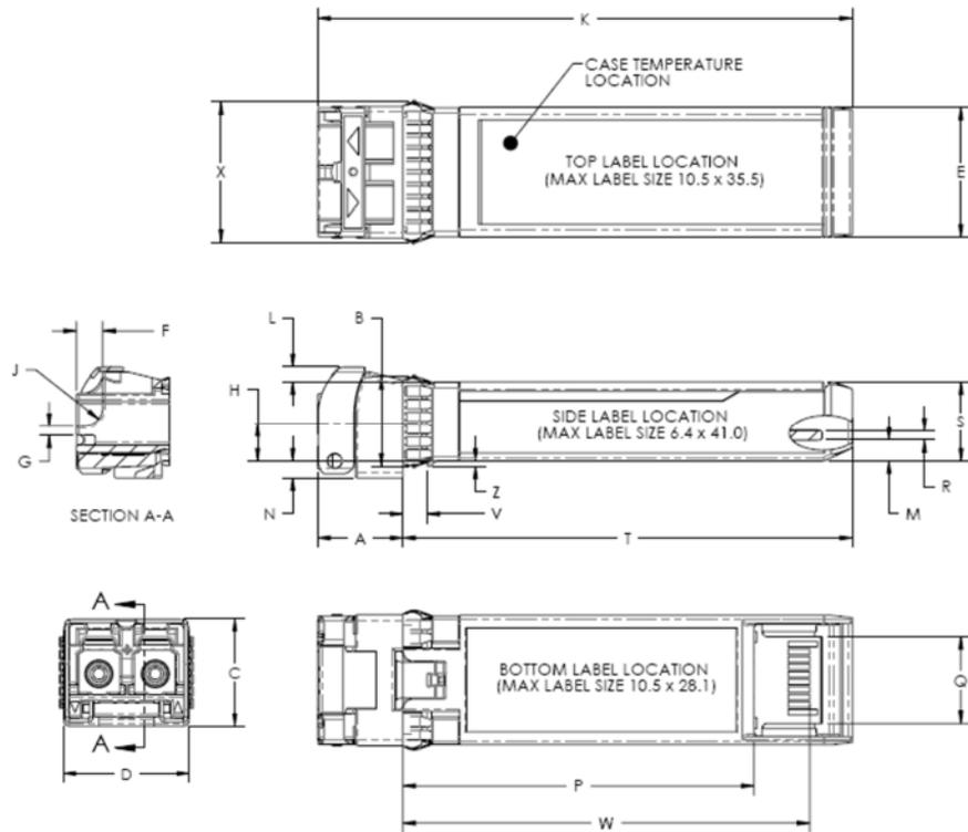
Figure 2. Mechanical Dimensions
