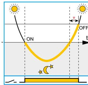
"Traditional" light dependent relays incorporate switching hysteresis to prevent malfunctioning or tripping. This results in an unnecessary delay in switching off, and a resulting waste of energy (over period T).
