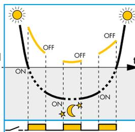
Incorrect functioning where the lamps cycle between On and Off, because their effect is being detected by the light sensor
