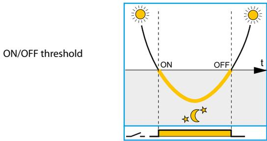
Switch OFF level = Switch ON level. Patented "zero hysteresis" circuitry ensures reliable switching without wasting energy.
