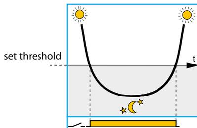
Correct functioning - provided the light sensor can be shielded from the effects of the controlled lighting switching On and Off
