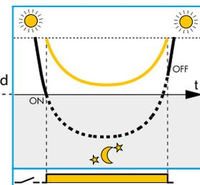
The innovative principle of "light feedback compensation" avoids the annoying and damaging effects of the lamps repeatedly "hunting" between On and Off, due to poor installation
