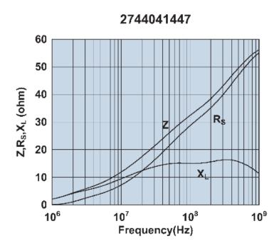
Impedance, reactance, and resistance vs. frequency.
