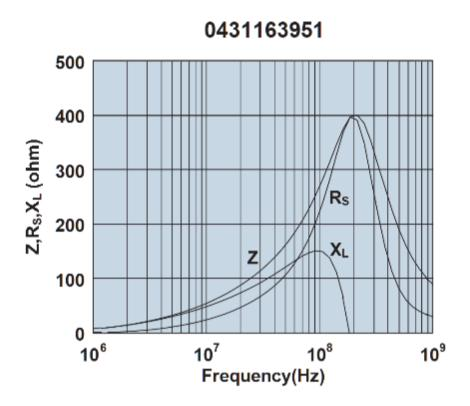
Impedance, reactance, and resistance vs. frequency.
