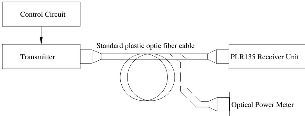
\*Fig.2 Measuring Method of Dissipation Current
