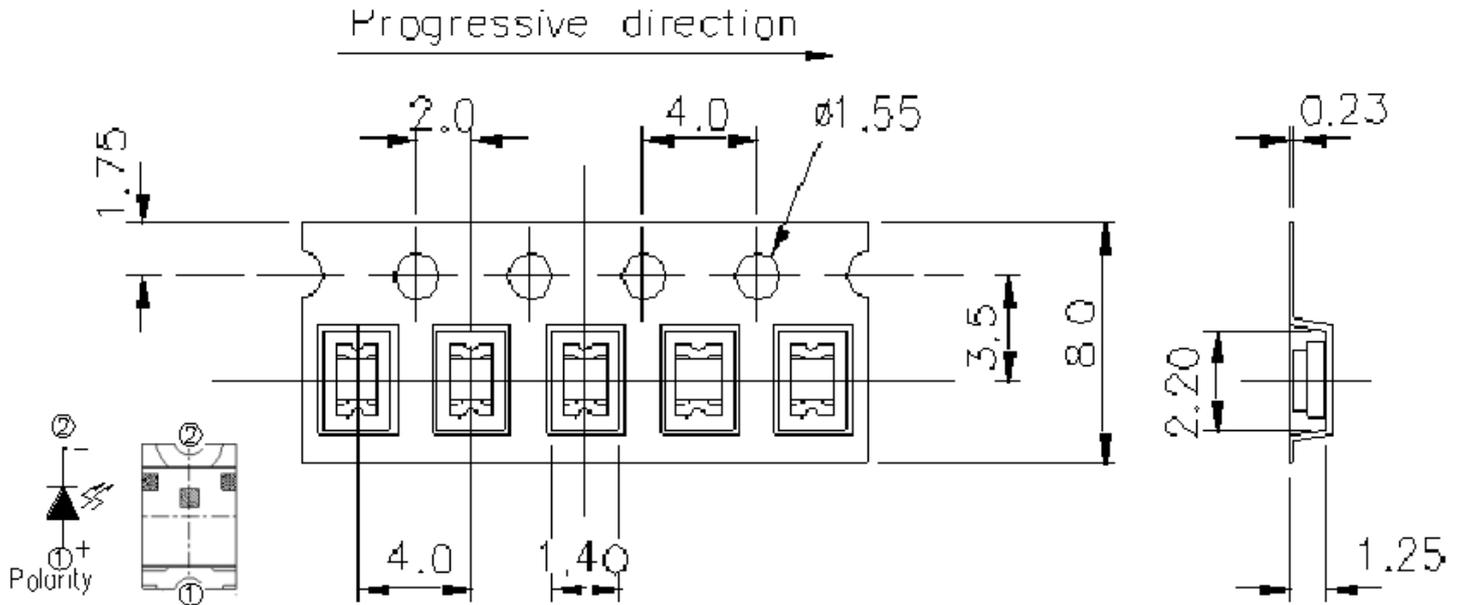
**Note:** The tolerances unless mentioned is  $\pm 0.1\text{mm}$ , Unit = mm
