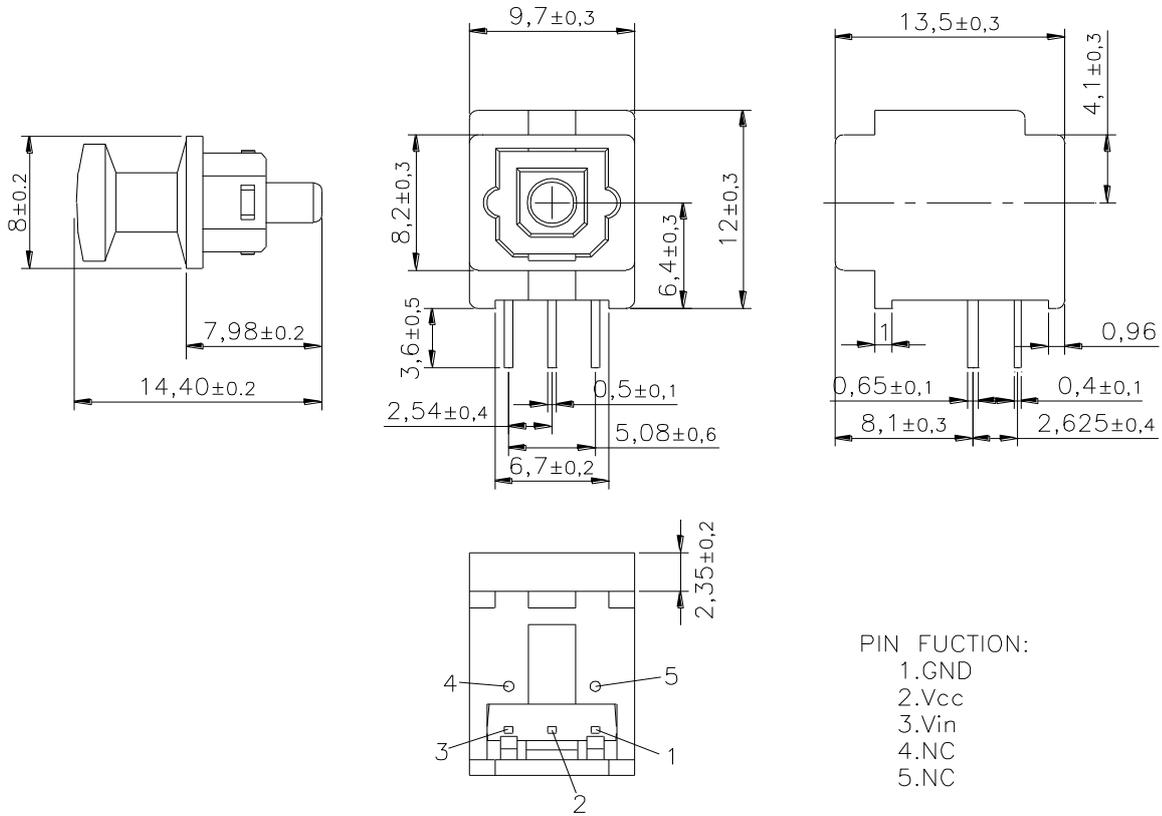
Note: Tolerances unless mentioned  $\pm 0.3$ mm. Unit = mm
