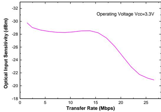
Note: Before using the EAPLR4A4 device, please confirm the minimum sensitivity at different operating voltage and transmission rate.
