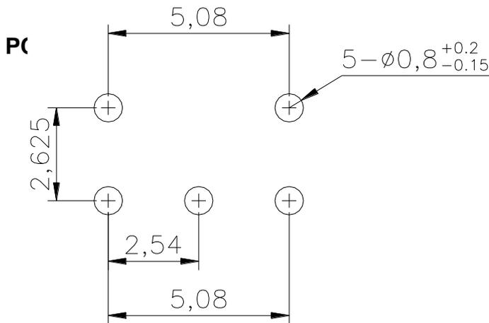
Note: PCB Tolerances: 1.6mm. Unit = mm
