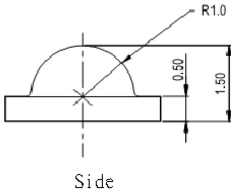
For reflow soldering (propose)
