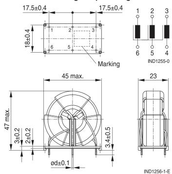
Part tolerances to ISO 2768-cL / ISO 8015. Size ISO 14405 (E) All dimensions in mm
