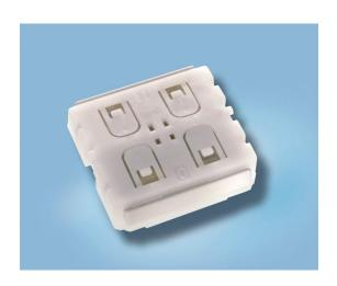
PTM 215 contains an additional encryption mode. Telegrams are encrypted via a combination of rolling code and AES128 encryption algorithm.
