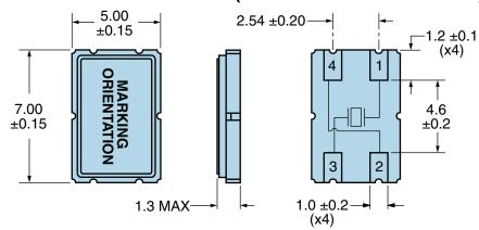
Note: Chamfer and index mark not shown.
