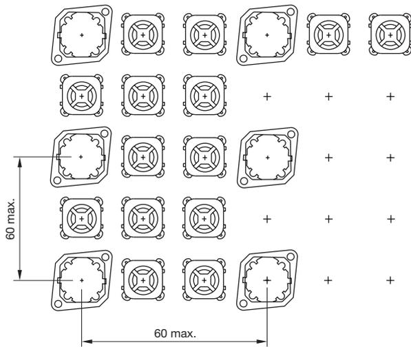
The arrangement of the mounting flanges and their number is determined by the size of the front panel or PCB. To ensure uniform, tactile switching, we recommend a layout of the flanges as per adjacent sketch.
