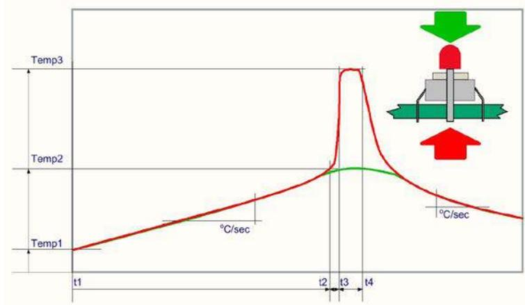
Green curve: Temperature on the component side of the pcb
