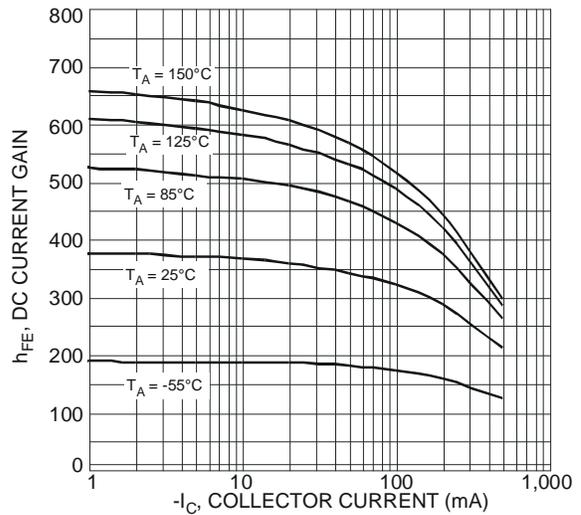
Fig. 5 Typical DC Current Gain vs. Collector Current
