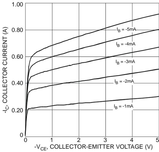
Fig. 4 Typical Collector Current vs. Collector-Emitter Voltage
