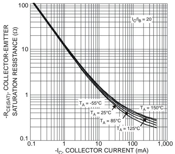
Fig. 9 Typical Collector-Emitter Saturation Resistance vs. Collector Current
