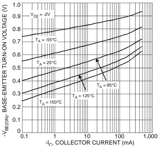
Fig. 8 Typical Base-Emitter Turn-On Voltage vs. Collector Current
