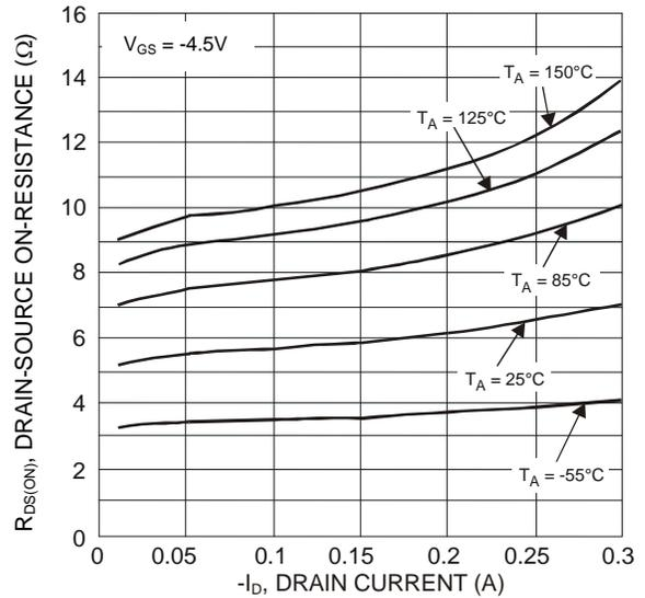
Fig. 4 On-Resistance vs. Drain Current and Temperature
