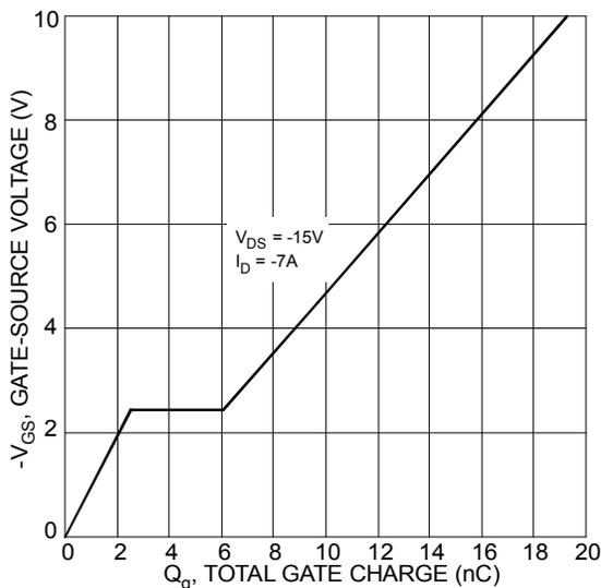
Figure 11 Gate-Charge Characteristics
