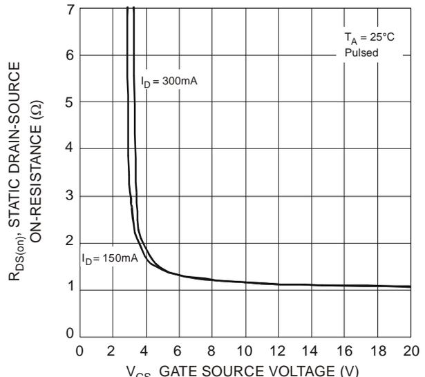
Figure 6 Static Drain-Source On-Resistance vs. Gate-Source Voltage
