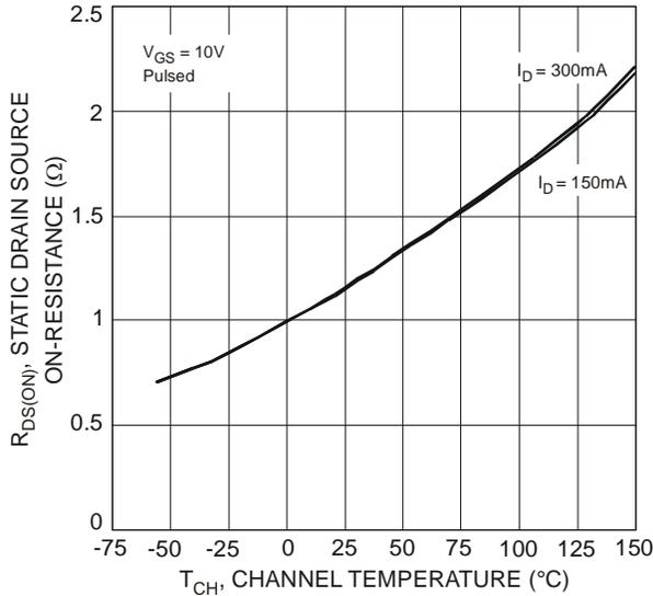
Figure 7 Static Drain-Source On-State Resistance vs. Channel Temperature
