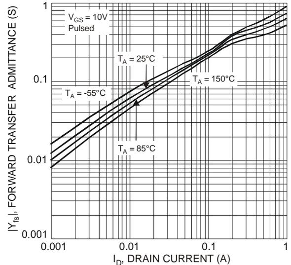
Figure 10 Forward Transfer Admittance vs. Drain Current
