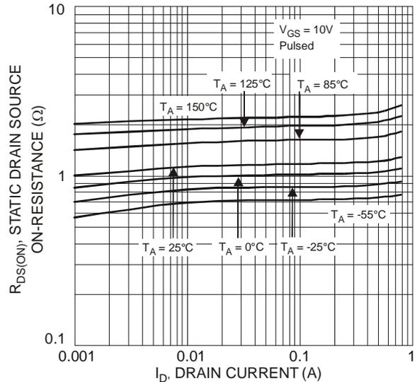
Figure 4 Static Drain-Source On-Resistance vs. Drain Current
