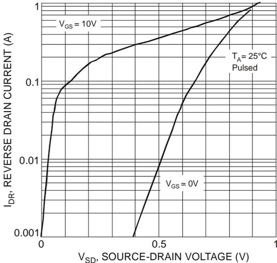
Figure 9 Reverse Drain Current vs. Source-Drain Voltage
