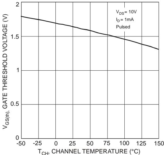
Figure 3 Gate Threshold Voltage vs. Channel Temperature
