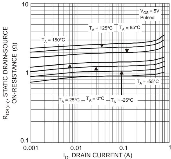
Figure 5 Static Drain-Source On-Resistance vs. Drain Current
