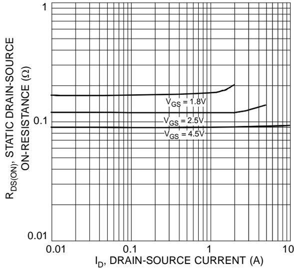
Fig. 3 On-Resistance vs. Drain-Source Current & Gate Voltage
