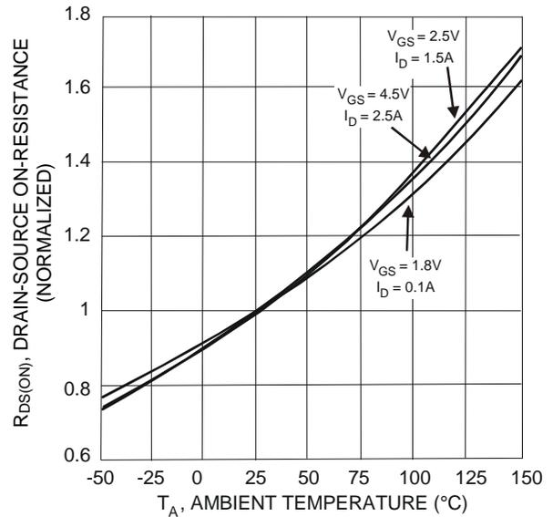
Fig. 4 Normalized Static Drain-Source On-Resistance vs. Ambient Temperature
