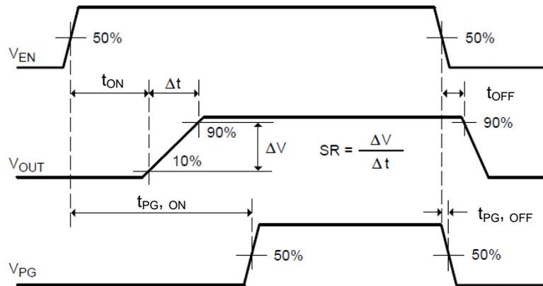
**Figure 1 Timing Diagram**
