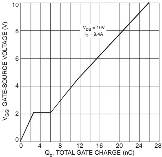
Fig. 11 Gate-Source Voltage vs. Total Gate Charge
