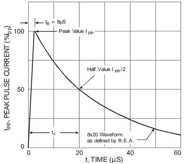
Figure 2 Pulse Waveform
