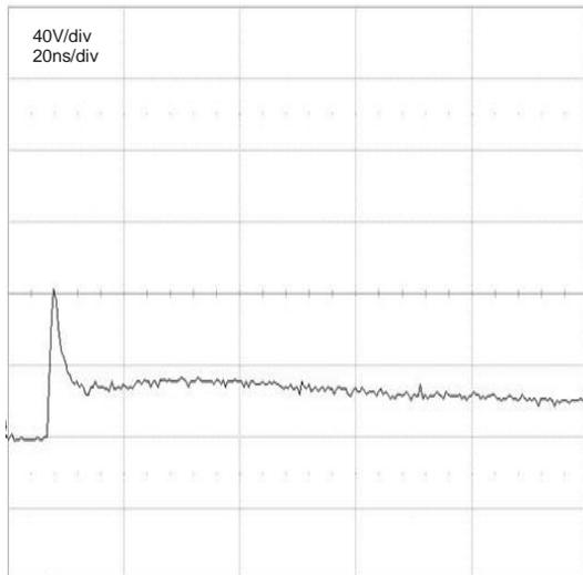
Figure 1 IEC 6100-4-2 Clamping Voltage
