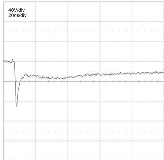
Figure 2 IEC 6100-4-2 Clamping Voltage
