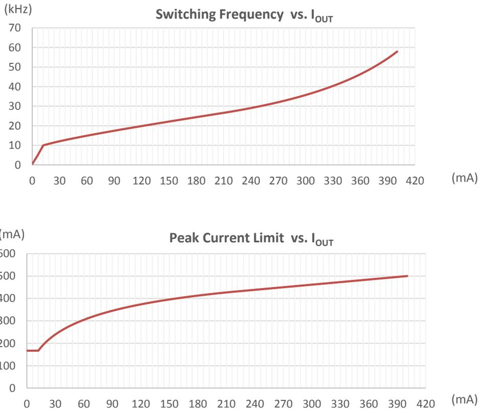
Figure 5. Frequency and Peak Current Limit Characteristic (Vo = 12V, L1 = 1mH)
