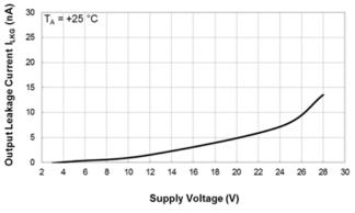
**Output Leakage Current vs Supply Voltage**
