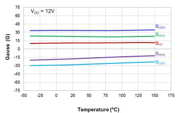
Switch Points B<sub>OPS</sub> and B<sub>RPS</sub> vs Temperature
