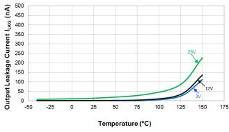
**Output Leakage Current vs Temperature**
