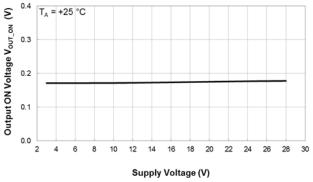
**Output ON Voltage vs Supply Voltage**
