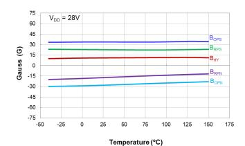
Switch Points B<sub>OPS</sub> and B<sub>RPS</sub> vs Temperature
