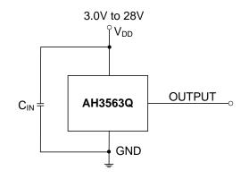
Note: 4. C<sub>IN</sub> is for power stabilization and to strengthen the noise immunity; the recommended capacitance is 10nF ~ 100nF.
