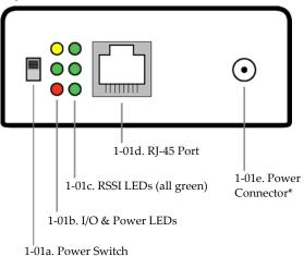
\* The Ethernet RF Modem does not support Power-over-Ethernet (PoE). The device cannot be powered directly from a PoE port on a compatible hub.
