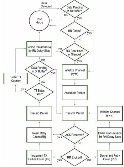
the effect of increasing the back-off delay, as the radio cannot return to RF transmit (or retransmit) mode as long as it is receiving RF data.
