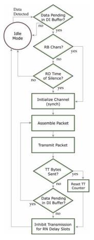
parameter is set to a non-zero value. These delays are intended to lessen congestion following long bursts of packets from a single transmitting modem, during which several receiving modems may have become ready to transmit.
