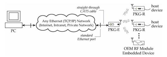
The Ethernet-connected RF modem supports com port and Telnet connection options:
