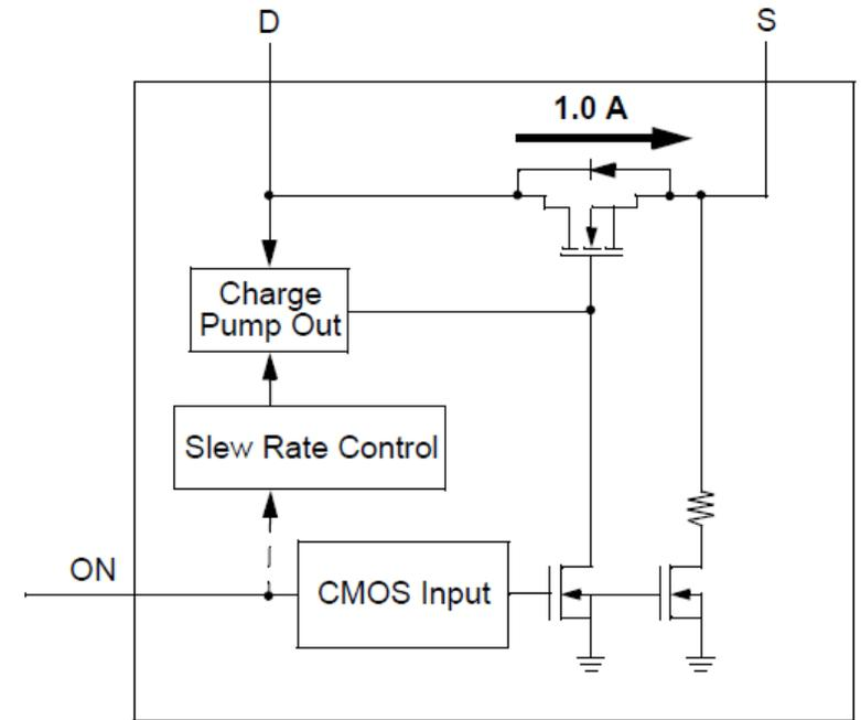
**Figure 1: SLG59M1466V Block Diagram**
