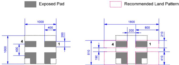
**Figure 2. SLG59M1466V Package Dimensions and Recommended Land Pattern**
