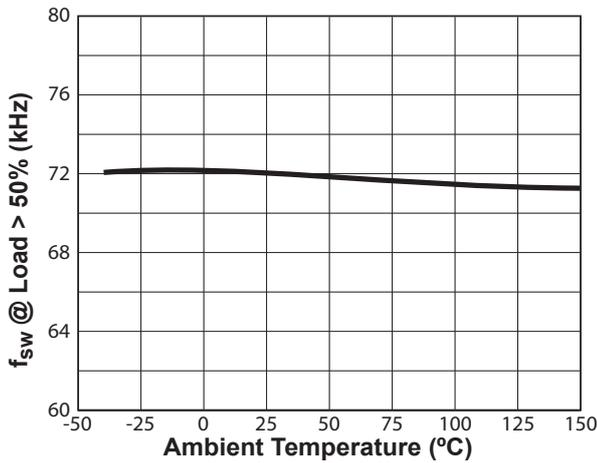
Figure 7.3 : Switching Frequency vs. Temperature<sup>1</sup>
