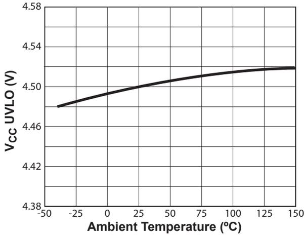
Figure 7.1 : V<sub>CC</sub> UVLO vs. Temperature
