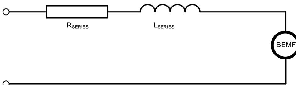
Figure 21: Equivalent Electrical Model of an Actuator
