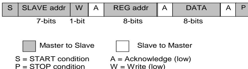
**Figure 35: I<sup>2</sup>C Byte Write (SDA line)**
