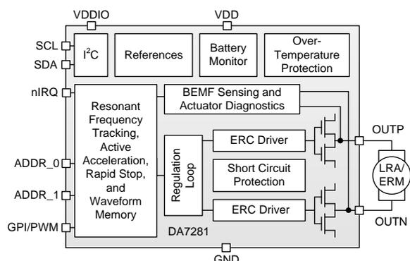
LRA/ERM Haptic Driver with Multiple I<sup>2</sup>C Addresses, Integrated Waveform Memory, and Wideband Support
