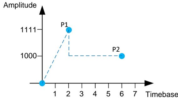
Figure 25: Snippet Ramp and Step with ACCELERATION\_EN = 1
