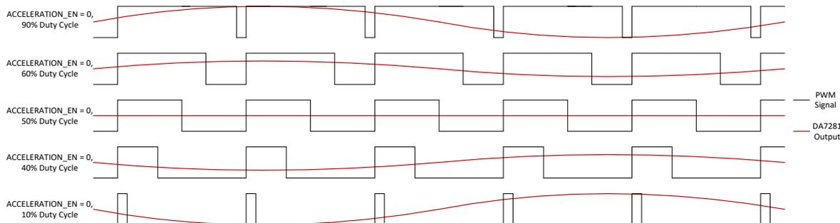
Figure 9: Example PWM Inputs with `ACCELERATION_EN = 0`
