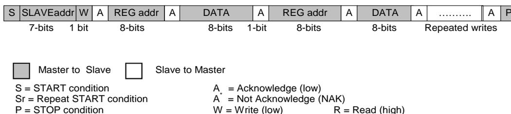
**Figure 39: I<sup>2</sup>C Repeated Write (SDA line)**
