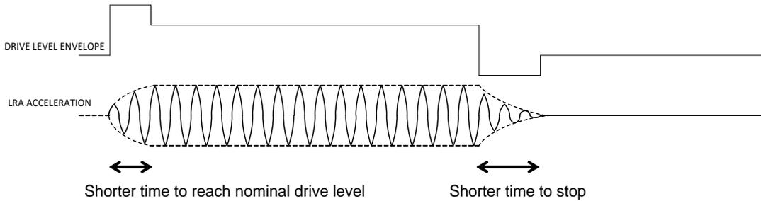
**Figure 11: LRA Single Step with Acceleration and Rapid Stop**
