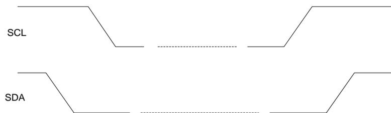
**Figure 34: I<sup>2</sup>C START and STOP Conditions**
