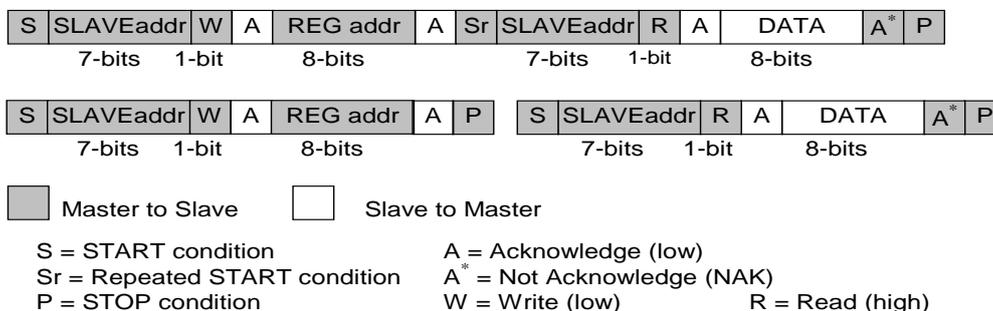
**Figure 36: Examples of the I<sup>2</sup>C Byte Read (SDA line)**
