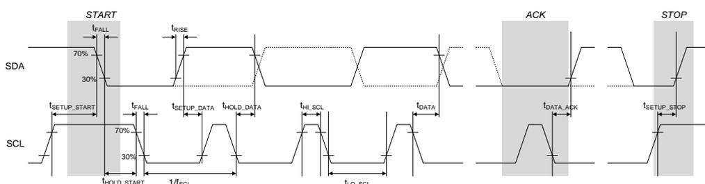
**Figure 4: I<sup>2</sup>C Interface Timing**
