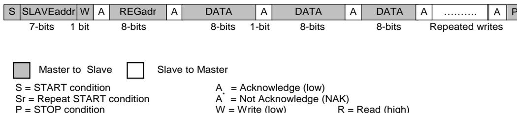
**Figure 38: I<sup>2</sup>C Page Write (SDA line)**
