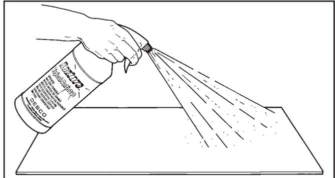
Figure 2. Applying Reztore™ Topical Antistat to the mat.
