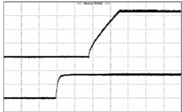
**Figure 7:** Turn-on transient at zero load current (5 ms/div). Vin=48V. Top Trace: Vout, 1.0V/div; Bottom Trace: ON/OFF input, 2V/div
