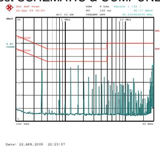
**Fig17: EMI test result** Vin = 48V Iout=20A AVERAGE
