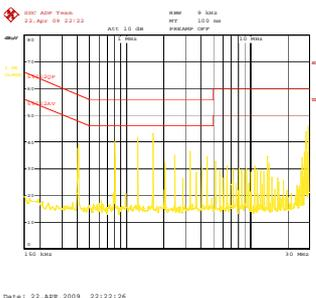
**Fig18: EMI test result** Vin = 48V Iout=20A Q.PEAK
