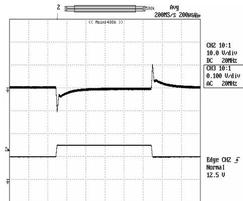
**Figure 9:** Output voltage response to step-change in load current (75%-50%-75% of Io, max; di/dt = 1.0A/μs). Load cap: 100μF tantalum capacitor and 1μF ceramic capacitor. Top Trace: Vout (100mV/div, 200us/div), Bottom Trace: Iout (10A/div). Scope measurement should be made using a BNC cable (length shorter than 20 inches). Position the load between 51 mm to 76 mm (2 inches to 3 inches) from the module
