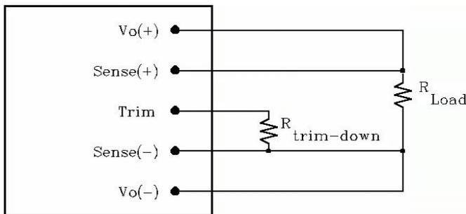
**Figure 21:** Circuit configuration for trim-down (decrease output voltage)
