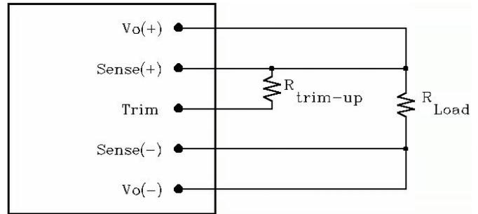
**Figure 22:** Circuit configuration for trim-up (increase output voltage)
