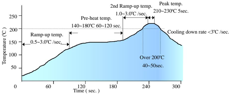
Note: The temperature refers to the pin of V48SR, measured on the pin +Vout joint.
