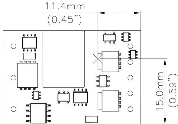
Figure 24: Temperature measurement location
