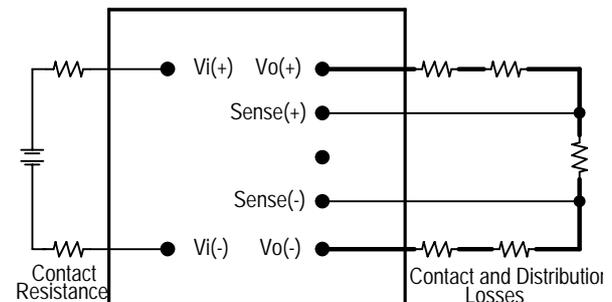
Figure 20: Effective circuit configuration for remote sense operation
