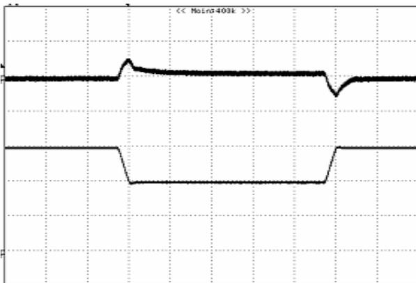
**Figure 8:** Output voltage response to step-change in load current (75%-50%-75% of Io, max; di/dt = 0.1A/μs). Load cap: 10μF tantalum capacitor and 1μF ceramic capacitor. Top Trace: Vout (100mV/div, 200us/div), Bottom Trace: Iout (5A/div). Scope measurement should be made using a BNC cable (length shorter than 20 inches). Position the load between 51 mm to 76 mm (2 inches to 3 inches) from the module
