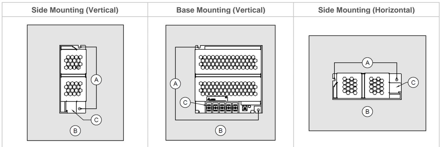
Fig. 2 Mounting Orientation
