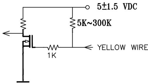
14-1. THE FAN SPEED WILL DEFAULT TO MAXIMUM WHEN THE SPEED CONTROLL INPUT IS LEFT UNCONNECTED.
