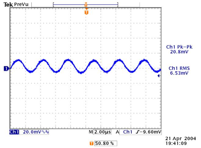
Figure 8: Output ripple & noise at 3.3Vin, 1.8V/10A out
