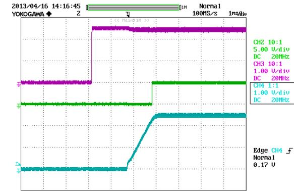
**Figure 16:** Turn on delay time at 12Vin, 2.5V/40A out (4mS/div)
