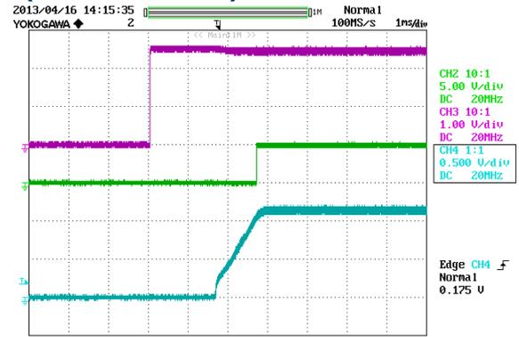
**Figure 14:** Turn on delay time at 12Vin, 1.2V/40A out (4mS/div)
