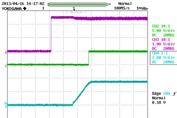
**Figure 17:** Turn on delay time at 12Vin, 3.3V/40A out (4mS/div)
