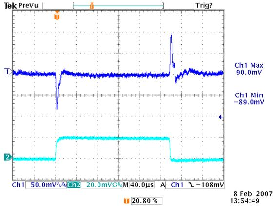
**Figure 19:** Transient Response at 12Vin, 0.9V/40A out (40uS/div)
