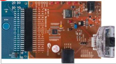
1. Connect the CY3280-SLM board to the CY3280-20x34 UCC board's P2 connector.
