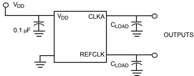
**Note:** All capacitors should be placed as close to each pin as possible.
