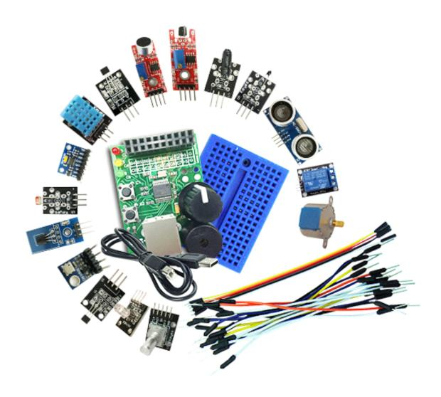
This product includes the E3mini Board and sensors shown below. The CD contains a C compiler and a PDF tutorial with example code for each sensor.
