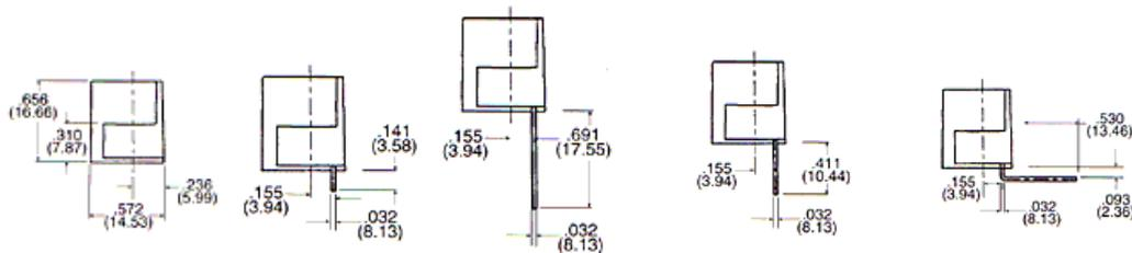
0 = Flush Mount    1 – PC Pin    2 – Wire Wrap    3 – Turret Type    4 – Right Angle PC Pin
