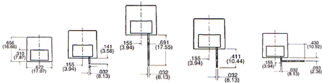
0 = Flush Mount    1 – PC Pin    2 – Wire Wrap    3 – Turret Type    4 – Right Angle PC Pin
