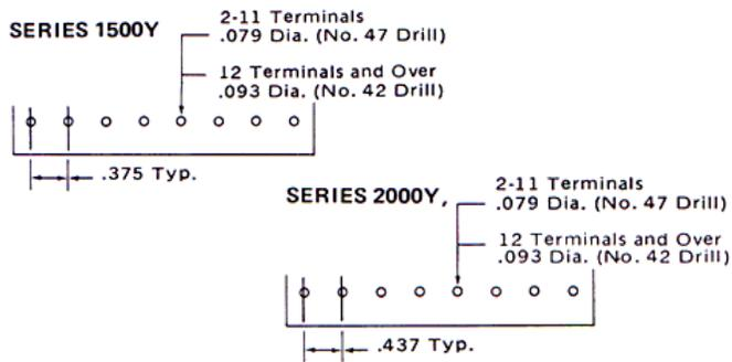
1500/2000 – Available with .187" x .020" quick-connect tabs for 1500 Series; .250" x 0.32" for 2000 Series. Nine styles ...tin-plated brass tabs held in place by terminal screws. Up to six terminations per pole. To order, specify:
